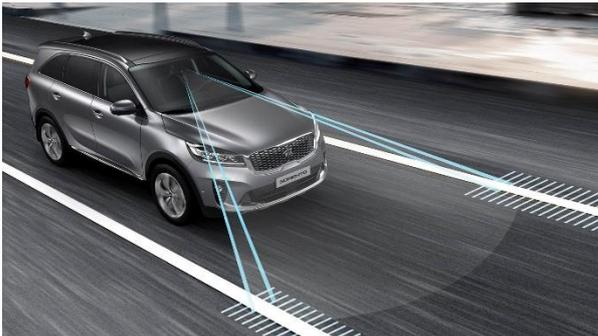
Figure 4. Illustration of camera detection used in Lane Keep Assist technology<sup>iv</sup>
